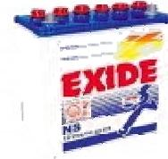
**Why it happened:** Instead of removing the ground (negative, black color) cable first, the Worker was removing the positive (red) cable with a wrench that simultaneously touched some other conductor and a **SPARK** occurred in the vicinity where **FLAMMABLE HYDROGEN GAS** was coming out of the battery. In the presence of **Air**, the three elements of a Fire Triangle i.e. 1. Fuel, 2. Source of Ignition, and 3. Air combined and an explosion occurred.
